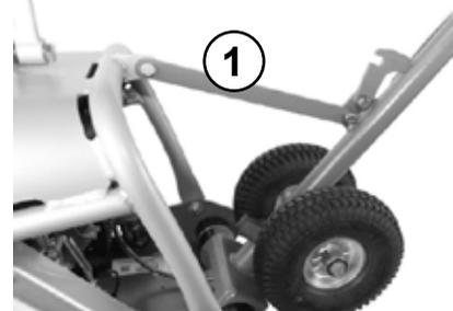
Tilt the machine to the rear and guide it via the guide bar.
